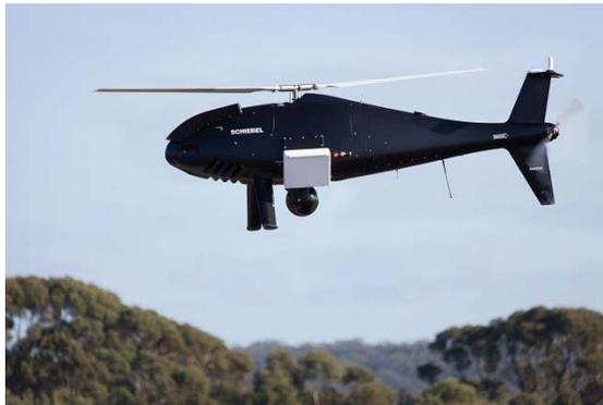
File picture by Schiebel: Camcopter during trials with the RAN fitted with Finmeccanica - Selex ES SAGE ESM and PicoSAR radar and the L-3 Wescam MX-10
