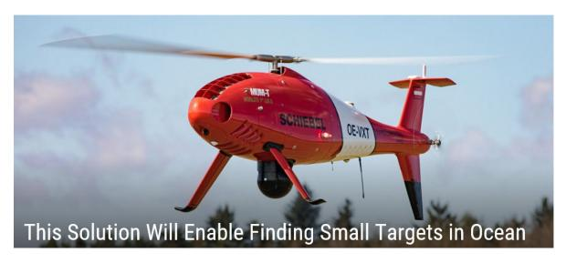
Whether searching for refugee boats at long range, enforcing fisheries protection rights, stopping drug runners, or rescuing people in water, patrol aircraft need all the tools they can get to find small targets in huge bodies of water. Schiebel and Overwatch Imaging successfully integrated PT8 Oceanwatch, a small target detection payload, on the CAMCOPTER S-100 Unmanned Air System.
