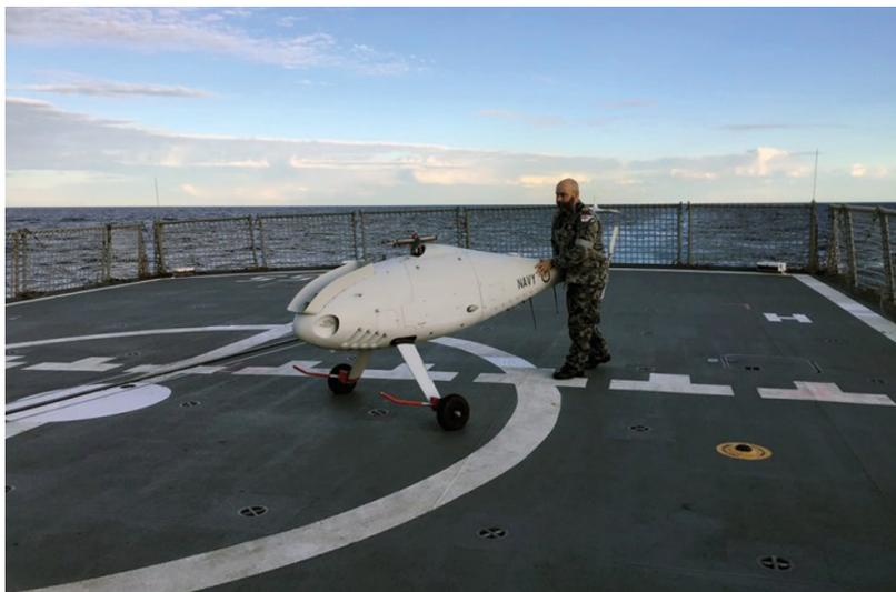
Two of Navy's newest cutting-edge capabilities have combined, with the Anzac Class Frigate HMAS Ballarat embarking an S-100 Camcopter Unmanned Aerial Vehicle for flight trials off the Eastern coast of Australia.
