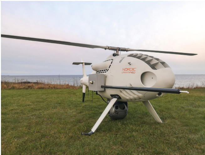
The CAMCOPTER S-100 can carry multiple payloads with a combined weight of up to 50 kg. Schiebel Group Photo
