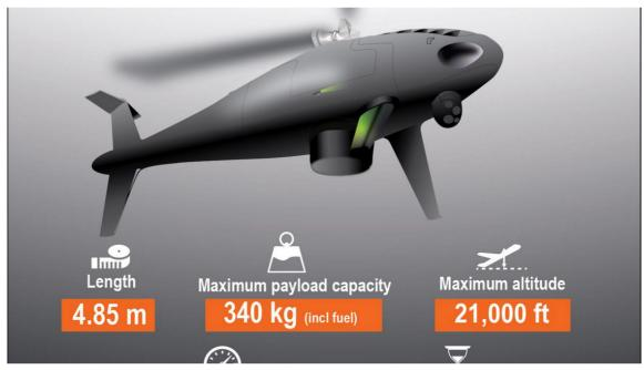
A model of Schiebel's Camcopter S-300 vertical take-off and landing (VTOL) unmanned aerial vehicle (UAV). Schiebel in collaboration with South Korea's Hanwha Systems and UI Helicopter will provide three Camcopter S-300s equipped with locally developed synthetic aperture radars (SARs) and electro-optical/infrared (EO/IR) sensors to the RoK Navy. (Janes)
